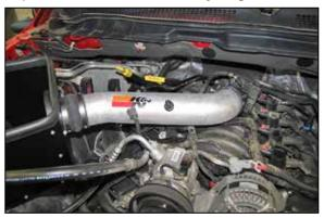
19. Install the K&N® intake tube into the coupler at the heat shield and then into the coupler at the throttle body. Adjust the tube for best fit and then secure with the provided hose clamp.
