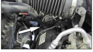
3. Disconnect the crank case vent hose from the valve cover fitting and then lift up and remove the air filter housing and intake tube to remove it from the vehicle.
