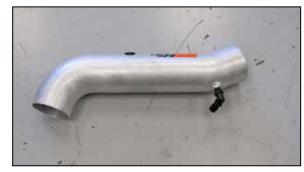
16. Install the 90° NPT fitting into the K&N $^{\mbox{\tiny 8}}$  intake tube as shown.
