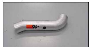
15. Install the provided grommet into the K&N® intake tube as shown.
