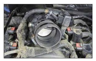
5. Install the provided coupling hose (08496) onto the throttle body and secure with the provided hose clamp.
