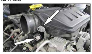
4. Disconnect the inlet air temperature sensor electrical connection and remove the bolt shown that secures the intake plenum. Lift up and remove the intake plenum from the vehicle.
