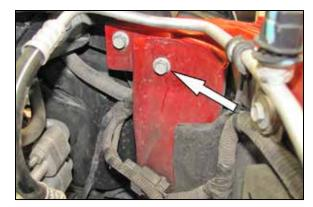
12. Remove the core support bolt shown.
