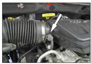
2. Loosen the hose securing the intake tube to the intake plenum.
